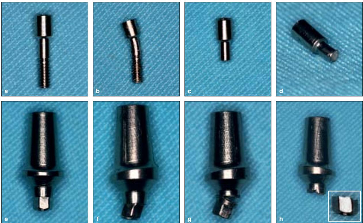
**Fig 3** Failure modes of group 3 specimens after mechanical testing: (a) intact screw, (b) screw bending, (c and d) screw fracture localized in the transition area from the smooth to the threaded surface, (e) intact abutment, (f) abutment bending, and (g and h) abutment partial and total fracture, respectively.
